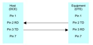
However, if the other end (Host side) is also a DTE, then a null-modem connector or cable is required. This effectively swaps pins 2 and 3.
