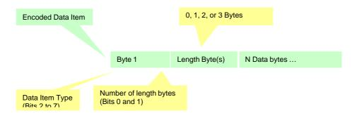
The following shows how an ASCII data item can be encoded. Depending upon how many data bytes it contains, it may require zero, one, two, or three length bytes to represent the total number of data bytes.
