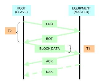
**RTY** – This defines the number of times to initiate the block transfer (start sending with the ENQ.) Upon the receipt of a NAK (or other protocol error), the RTY value is adjusted and the block transfer is again attempted.
